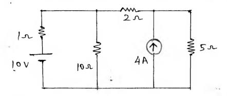
3a For the circuit given below determine  $R_L$  for maximum power transfer. Also calculate the maximum power.
