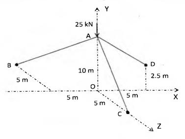
Q.4 (a) Find the forces in all the members of the truss loaded as shown in figure below. (12)
