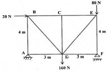
Q.4 (b) A truss is loaded as shown in figure below. Find force in members BC and EF of (08) the truss by method of sections only.
