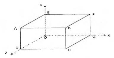
Q.3 (b) A vertical load of 25 kN is supported by three bars of a tripod as shown in figure (10) below. Find the forces in each bar. Note that points B and C lie in XZ plane.
