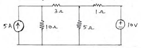
c Determine the current through the 10 ohm resistor using superposition theorem.
